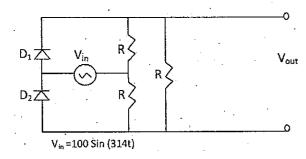
Determine  $v_0$  for network given below.
